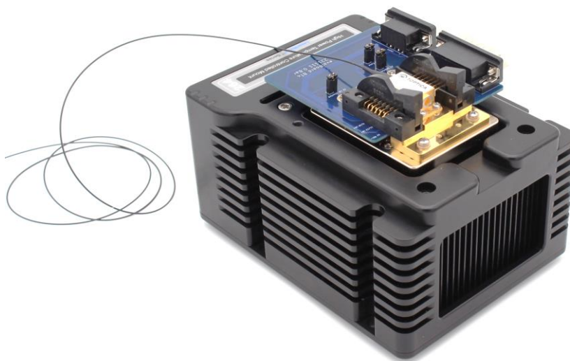
Figure 5 Evaluation Board at Arroyo 264-BB LaserMount
