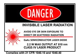
The laser emission from this diode is close to the invisible infrared region of the electromagnetic spectrum. Avoid direct and/or indirect exposure to the free running beam. Collimating the free running beam with optics as common in optical instruments will increase threat to the human eye.
